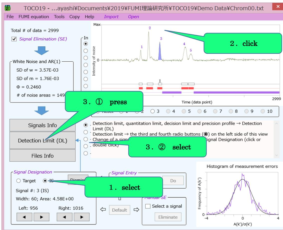
Figure 13 --- The main window after an IS peak has been selected
