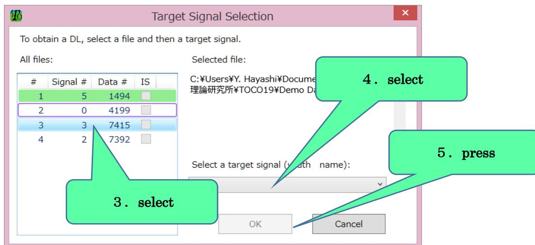
Figure 7 --- Target Signal Selection dialog box
