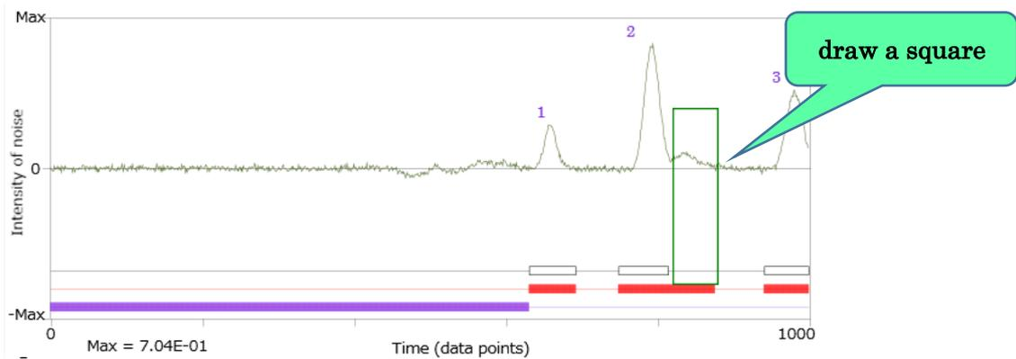
Figure 25 --- Another example of separation of overlapping peaks
